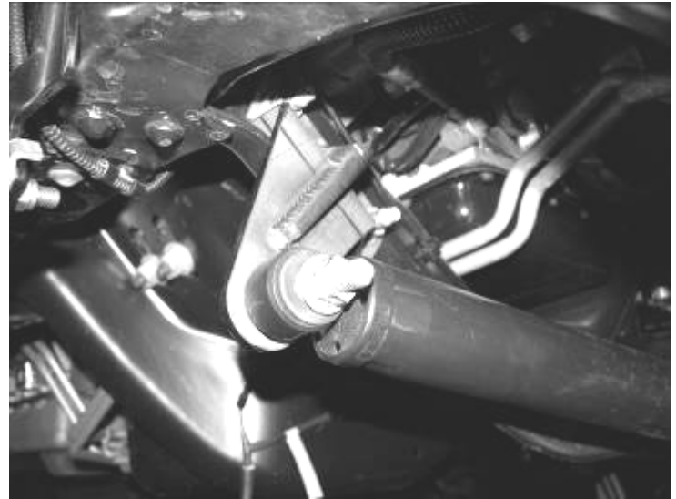
Picture Shown with Factory Stabilizer re-installed
