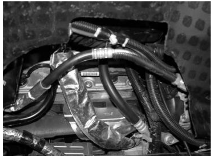
Photo shows bent A/C line
