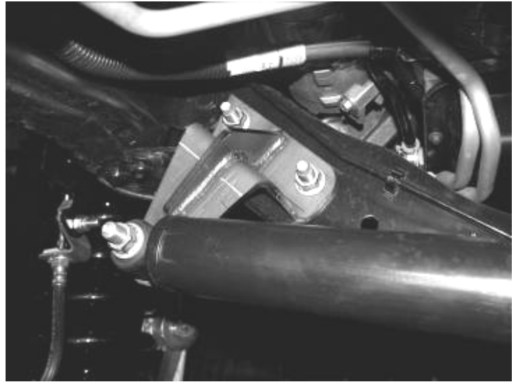
Picture Shown with Factory Stabilizer re-installed
