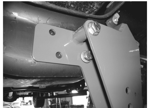
Driver Side I-beam Bracket FT410-104 Viewed from the front
