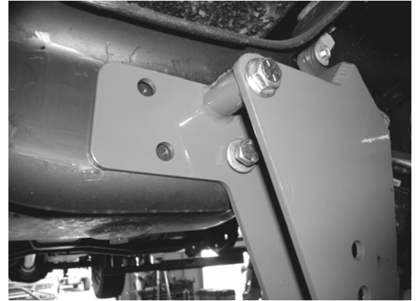
Driver Side I-beam Bracket Passenger I-Beam connection point
