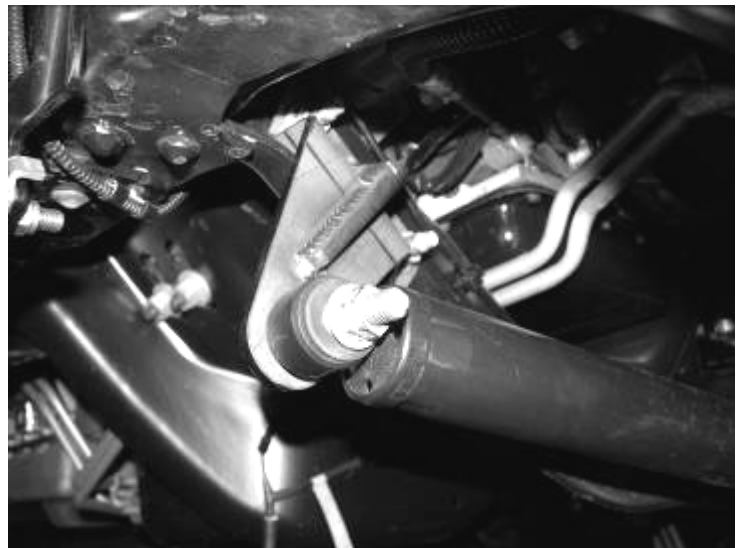
Picture Shown with Factory Stabilizer re-installed
