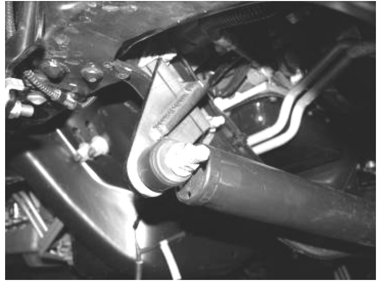
Picture Shown with Factory Stabilizer re-installed
