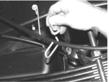
Clamp the leaf spring in the middle of the spring and remove the center bolt. (DO NOT REMOVE THE LEAF SPRING FROM THE TRUCK)
