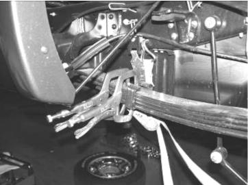
4. Separate the individual leafs and install the provided FT30275 add a leafs with the new center bolt in a pyramid pattern smallest on the bottom graduating to the longest on top. Locate FT30284 Leaf Spring Spacer and place on the bottom of the stack. Clamp the spacer and springs and tighten the center bolt as not to leave a gap between the springs. Cut the thread of the bolt smooth with the nut. The nut should be on the top of the leaf spring pack. SEE DRAWING ON NEXT PAGE
