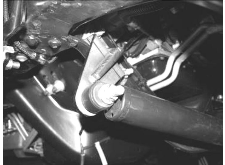
Picture Shown with Factory Stabilizer re-installed
