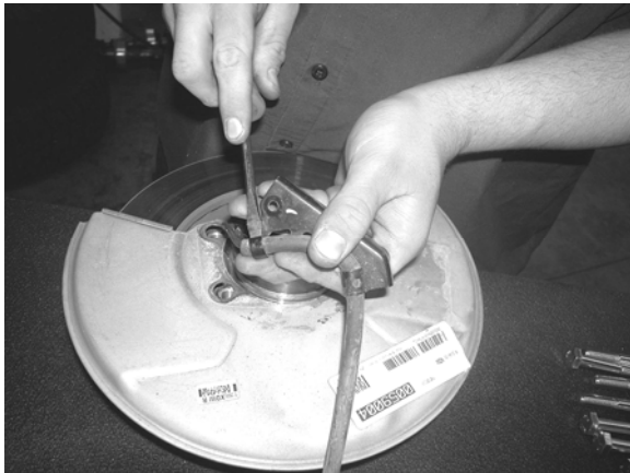
picture shown removing ABS line bracket
