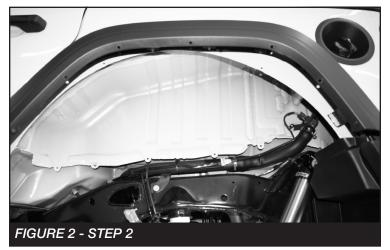
Release the (11) white clips attaching the fender to the body panel then remove the fender from the vehicle. SEE FIGURE 3-4
