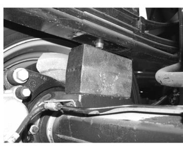
4. Install Fabtech Performance Shocks or Dirt Logic Shocks (not included) with the factory hardware and torque bolts to 65lbs.
