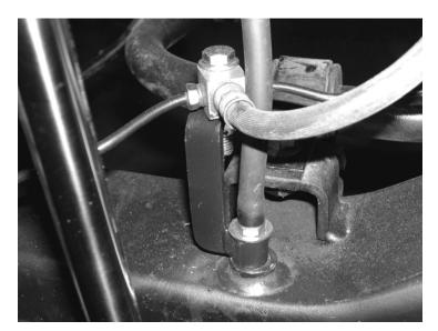
3. Locate the supplied rear lift blocks. Drill the hole in the top of the block out to 3/4". Insert the supplied FT178 Block Pin Sleeve into the axle perch. Install the provided lift blocks with the short center pin of the block facing down to the axle. Using the supplied u-bolts, nuts, and washers align axle, lift blocks, and springs and torque to U-Bolts to 296lbs. SEE PHOTOS BELOW.
