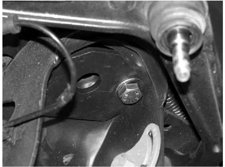
37. Install the upper shock mount (FT20484) into the factory upper shock tower using the using two 9/16"-12 x 1-1/4", washers and lock nuts. Torque to 184 ft-lbs. NOTE: Using a grinder, open up the hole on the upper factory shock mount to prevent contact with the new Fabtech upper shock washer. SEE PHOTO BELOW
