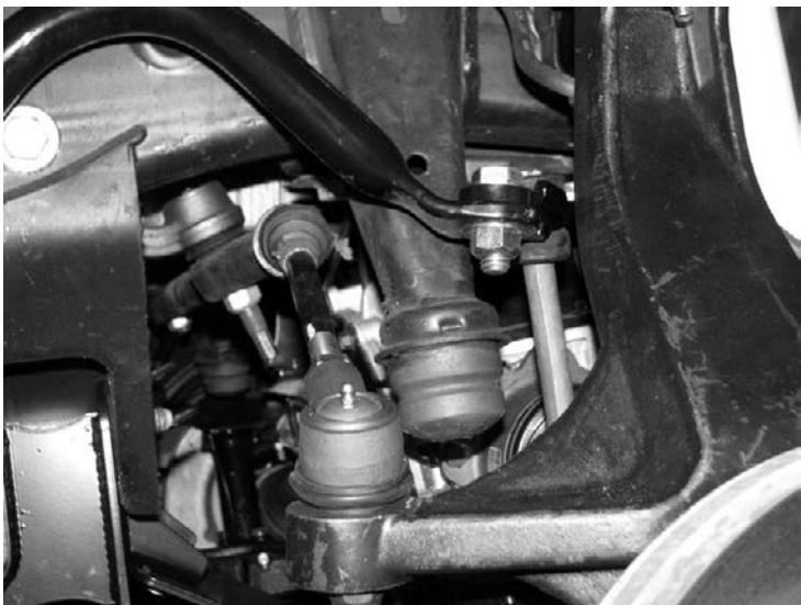
47. Install the front brake line extension bracket (FT20520) with the factory hardware and supplied 5/16" hardware. Clamp the ABS and brake line to the spindle using the supplied adel clamps and 1/4" bolts. SEE PHOTOS BELOW
