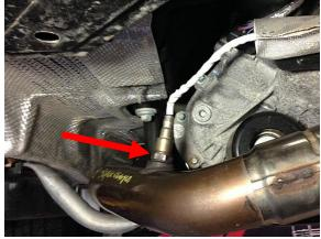
4. Remove the mounting bolts from the exhaust manifold flange.
