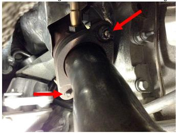
5. At this point you will be able to remove the factory downpipes. It is not necessary to remove the rear section of the exhaust. There is enough play in the exhaust hangers to allow removal of the downpipes.
