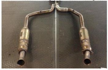
6. You are ready to install your new Fabspeed Sport Cat exhaust. Install the system in the reverse order used when removing the factory downpipe system. Use supplied hardware to mount exhaust manifold flange.
