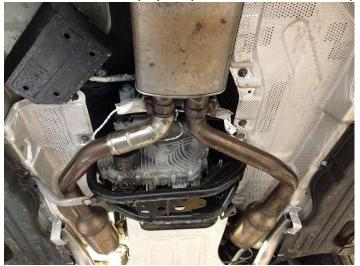
2. Loosen factory clamps connecting downpipe to center resonator.
