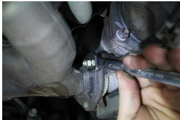
3. Using a 13mm socket, remove the (9) bolts securing each header to the engine block. (NOTE: *Break these bolts loose by hand. Do NOT use an electric or pneumatic impact wrench, as it can shear the bolts and damage the engine block.*)
