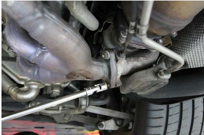
2. Remove any remaining turbo studs from the right side turbo by threading two 13mm nuts against one another and using a wrench to spin the stud out from the inner-most nut. (NOTE: *13mm nuts are available at all major hardware stores.*) Due to the angle of the left side turbo, it is not necessary to remove the studs. (*If they come out in the process, it is not a problem.*)
