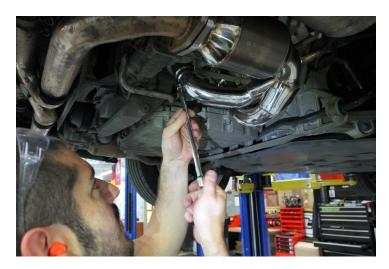
9. Insert the (3) supplied bolts and nuts into the muffler flange and tighten using a 13mm wrench and socket.
