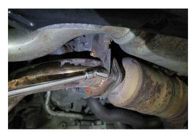
3. Pry back the side muffler brackets using a pry bar or a flat-head screwdriver.
