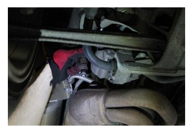
2. Using a 13mm socket, remove the (3) nuts securing the cats to the muffler inlets.
