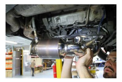
8. Re-insert the (9) flange bolts to secure the headers to the engine block.
