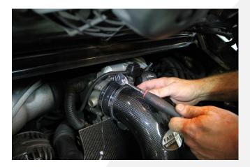
18. Re-connect mass airflow sensor plug.
