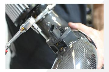
12. Using the supplied screw, attach the heat shield support bracket to the threaded boss on the engine as indicated.
