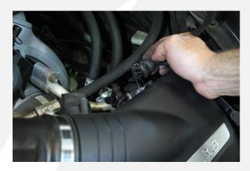
5. Unclip solenoid from the rear of the air box.
