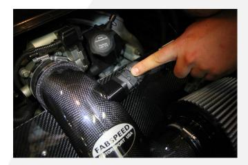
19. Re-connect vacuum hose and electrical connector to the solenoid as shown.
