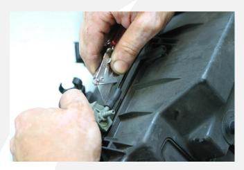
8. Disconnect solenoid from the remaining vacuum line and remove from the air box.
