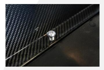
16. Attach the heat shield to the installed bracket using the supplied Allen/hex-head screw & nut.
