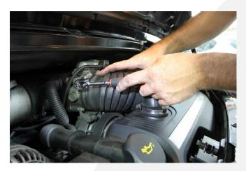
3. Disconnect the mass airflow sensor plug from the back of the air box.
