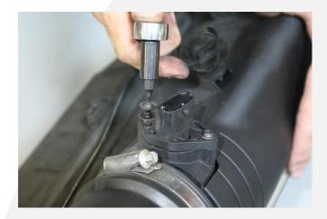
10. Remove the mass airflow sensor.
