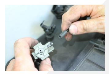
9. Using a T-20 "Tamper-Proof" Torx, loosen and remove the (2) screws securing the mass airflow sensor to the factory air box.
