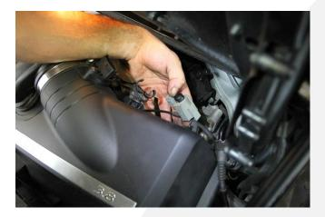
6. Disconnect the vehicle vacuum line from the nipple on the solenoid.
