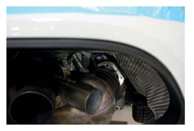
11. Using a 22mm wrench, remove both of the O2 sensors from each cat.
