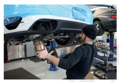
**NOTE:** After removing factory exhaust, visually inspect the threads on the turbo studs. If necessary, re-chase the thread with an 8x1.25 thread die.
