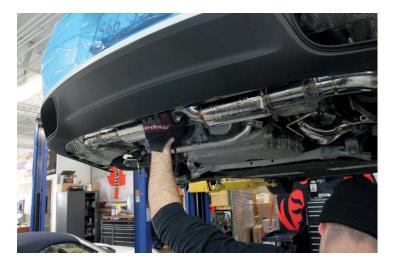
17. Position the right side of the assembly up onto the turbo studs, installing the factory turbo heat shield in the process. Finger tighten (4) flange nuts to hold the system in place.
