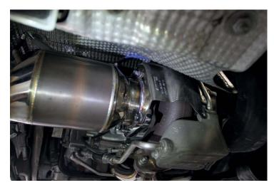
18. Using a 12mm wrench, tighten the (4) flange nuts on either side.
