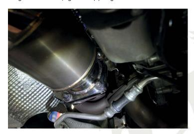
19. Using a 14mm wrench, re-install and tighten the EGT sensor on each side.
