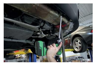
9. At this point, the muffler and the attached catalytic converters will be free from the car. If necessary, use a flat head pry bar to gently break the seal between the cats and the turbos.
