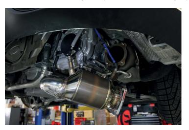
15. Slide the right side cat into the right side of the x-pipe. (Be sure that you have an Accuseal clamp slid on to the x-pipe.)
