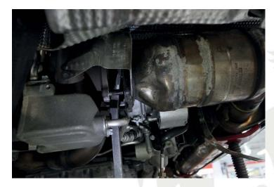
10. With the muffler supported, lower the exhaust slightly so that the O2 sensors can be accessed through the outlet opening in the rear bumper.
