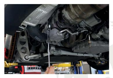
7. Using pole jacks, support the main section of the factory muffler.
