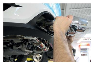
24. Align tips as desired and tighten Accuseals with a 15mm socket.
