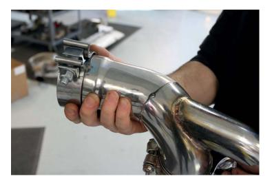
23. Position tip through opening in rear bumper and slide onto the open end of the x-pipe.
