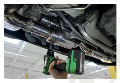
22. Slide an Accuseal clamp onto the tip inlets.
