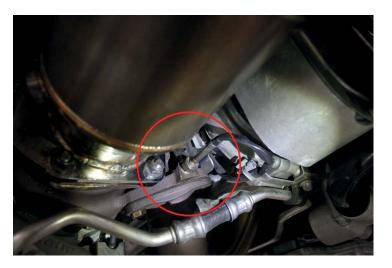
20. Check positioning of x-pipe to be sure that the unit is centered between the cats and it is rotated flat against the factory muffler bracket. Tighten Accuseal clamps using a 15mm socket.
