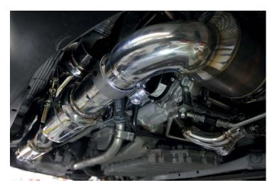
21. Slide supplied band clamps over the x-pipe and position in place over the factory muffler brackets. Tighten clamps using 13mm deep socket.
