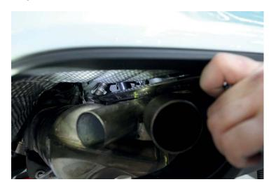
12. Remove pole jacks and lower muffler and cat assembly from the vehicle. (It may take some maneuvering to get this assembly out from the rear bumper due the very tight tolerances. Be patient!)
