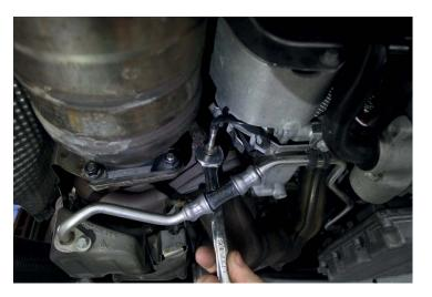
5. With the EGT sensors out of the way, use a 12mm wrench to loosen and remove the (4) flange bolts on each catalytic converter.
