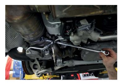
6. Using an 8mm wrench, loosen and remove the bolt securing the turbo heat shield on each side.
