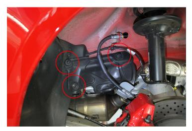
3. Loosen – *but do not remove* – (3) flange nuts.
