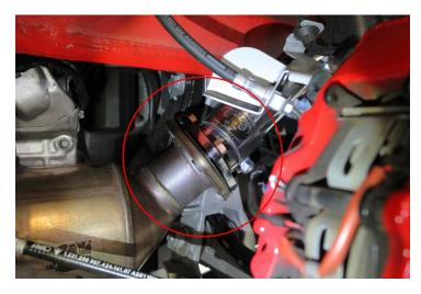
11. Assemble center section of Fabspeed system by connecting center slip joints and slide remaining band clamp on.
