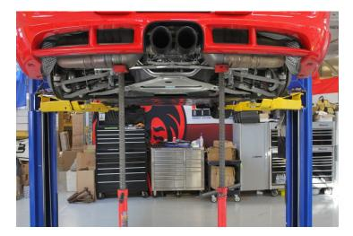
5. Remove loosened flange nuts.
