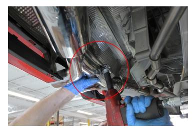
18. Tighten remaining band clamp over the center slip joint on the inlet tubing.
