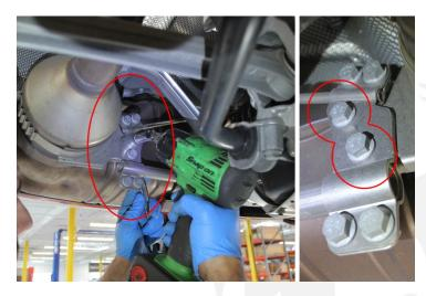
7. Lower and remove factory exhaust.
