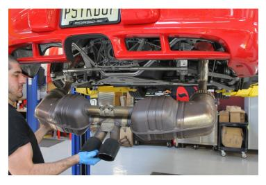
8. Assemble slip-joint sections of Fabspeed tubing and slide band clamps on.
