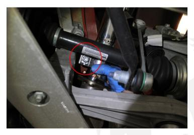
16. Tighten bracket bolts until snug; do not over-tighten, as crushing the vibration dampening gasket may cause damage.
