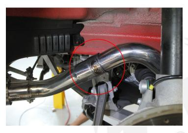
19. Position Fabspeed outlet tips on the center section outlet pipes and tighten mounting bolts.
