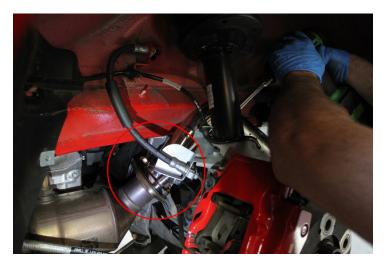
15. Position and tighten band clamp over the slip joint closest to the flange.
