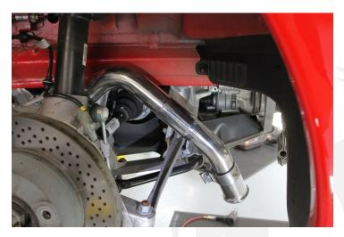
10. Hand tighten flange nuts; leave loose enough to re-position.
