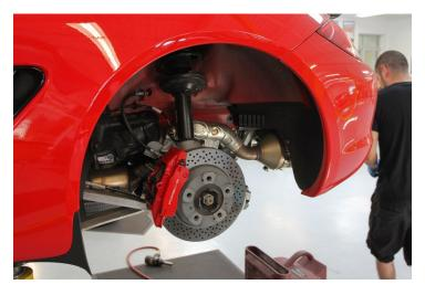
2. Remove (3) fasteners holding plastic cover inside rear wheel wells and remove cover.
