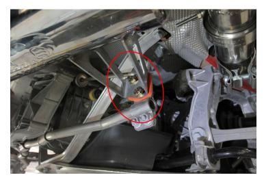
17. Verify alignment of both sides and tighten center section band clamp.
