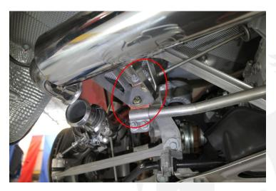
13. Apply and tighten v-band clamp to join the Fabspeed center section to the inlet tubing.
