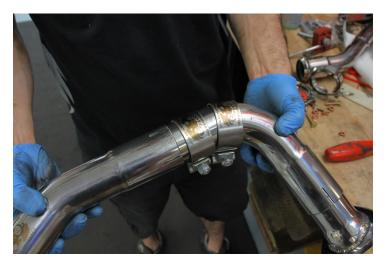
9. Position Fabspeed tubing and slip flange onto factory flange bolts.
