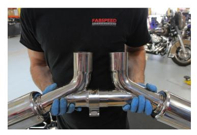
12. Position Fabspeed center section on vehicle and hand-tighten bracket bolts.
