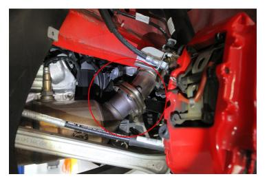
6. Remove (2) bolts from each side of the muffler hanger brackets.
