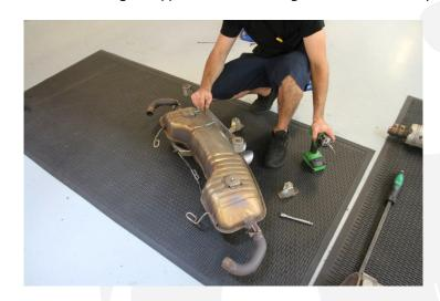
12) Attach provided muffler support bracket to factory upper muffler mounting bracket using 13mm bolt and 6mm Allen fasteners.
