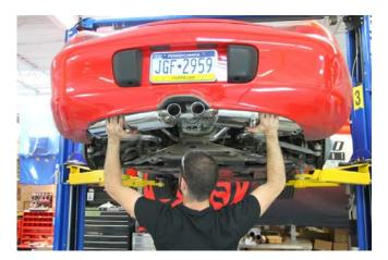
19) Line up connection between Maxflo mufflers and inlet pipes and attach with the provided v-bands clamps.
