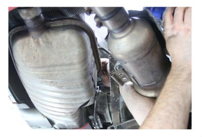
8) Lower and remove factory muffler from the vehicle.
