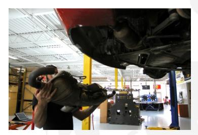
9) Remove (3) 13mm nuts and bolts from the flange connecting the inlet pipe to the header.
