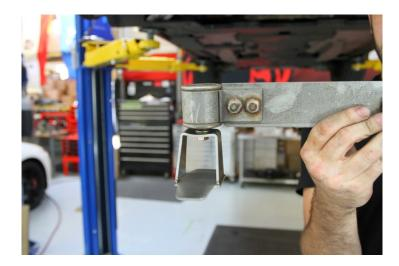
13) Re-attach upper center mounting bracket with Fabspeed mounting bracket attached, using the 13mm factory bolts that were removed in step 7.
