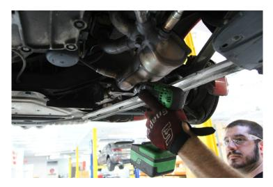
10) Remove secondary catalytic converters from the vehicle.
