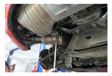
4) Loosen (2) 13mm sleeve clamps on both sides and slide the clamps out of the way.
