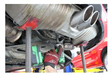
7) Remove (2) 13mm nuts from upper center muffler mounting bracket located in the center of the vehicle above the transmission. See photo in step 13 for bolt location. *NOTE: Keep these bolts for reinstallation.*
