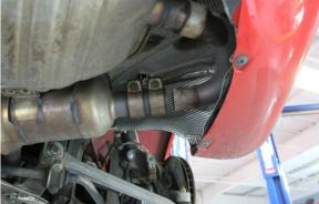
5) Support muffler as a safety precaution while unbolting it from the rear of the vehicle.
