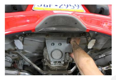
14) Identify left and right inlet pipes and position in vehicle.
