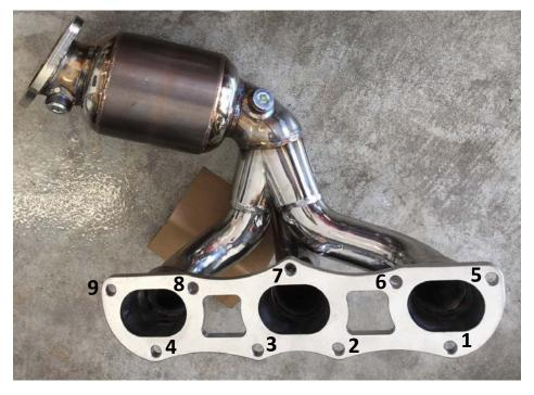
Screw heads in positions 2,3,5, and 9 should be readily accessible using the standard E12 socket and 3/8" extensions. Positions 6 and 8 should be easily accessible using a swivel connector. Positions 1,4,
