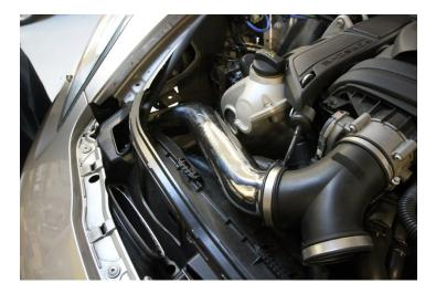
15. Re-insert and tighten the 10mm bolt through the bracket on the Fabspeed tube.
