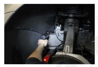
4. Remove left-side fender liner and repeat process to remove right-side fender liner.
