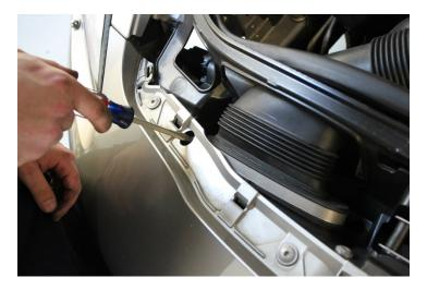
9. Separate the hoses from the factory intake y-pipe.
