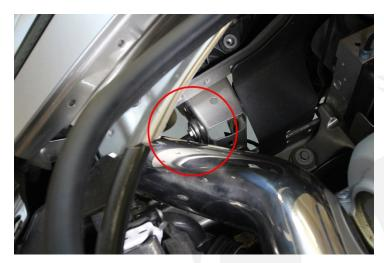
16. Tighten hose clamp to secure the Fabspeed tube into the factory y-pipe.
