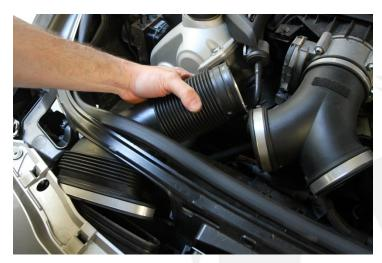
10. Remove factory intake tubes.
