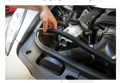
7. Separate and remove the front plastic trim panel at the front of the engine bay.
