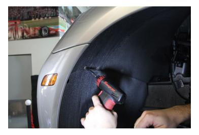
3. Remove the 10mm hex bolt securing the innermost tab of the fender liner.
