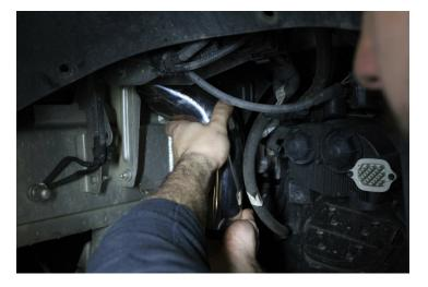
14. Fit the top end of the tubing into the factory y-pipe.
