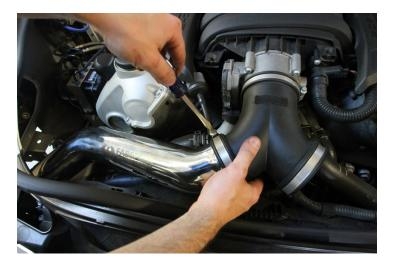
17. Re-install Fabspeed air filter on the bottom end of the intake tubing inside the right-side wheel well and tighten the hose clamp.
