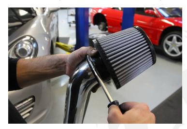
13. Insert the right-side Fabspeed intake tube through the opening in the wheel well.
