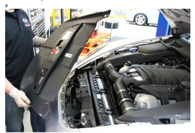
3. Open plastic cover near passenger side firewall and remove additional press-fit fastener.
