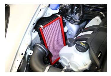
12. Replace factory airbox and re-fasten (2) metal clamps.
