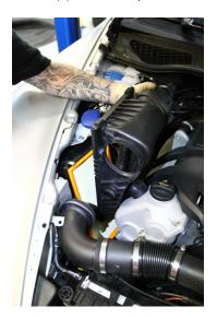
11. Remove factory/existing air filter and replace with new BMC filter.
