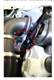
10. Release (2) metals clamps and remove passenger side airbox cover.
