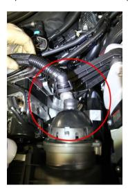
9. Separate smaller hose below the primary intake hose on the passenger side airbox.
