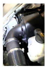
14. Re-insert and tighten (2) half-turn bolt fasteners.
