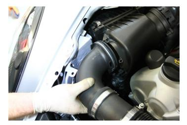
8. Separate smaller hose from rear of passenger side airbox.
