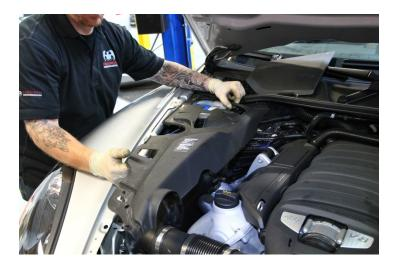
5. Remove press-fit fastener near driver side firewall and remove/set aside the driver side plastic cover.
