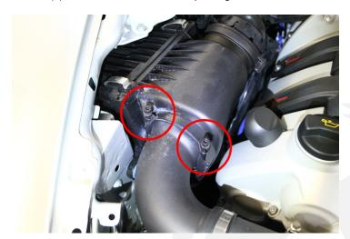
7. Separate primary intake hose from passenger side airbox.
