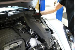
6. Remove (2) half-turn bolt fasteners from passenger side airbox cover.
