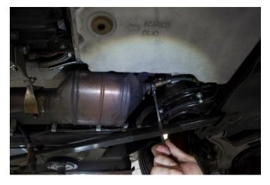
5. Loosen and remove the (3) flange nuts securing the factory cats.
