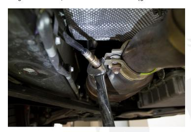
4. Remove the front oxygen sensors.
