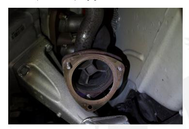
10. Align Fabspeed Sportcats and finger-tighten flange nuts.
