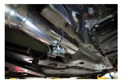
12. Install provided brackets by sliding tab (facing the front of the car) beneath the clamp and bolting to the bell housing.
