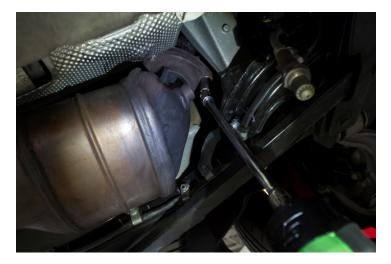
6. Loosen and remove the factory clamp securing the cats to the underside of the bell housing.
