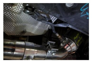
17. Remove the unused cable clip and re-fasten the remaining clip to secure the oxygen sensor cable.
