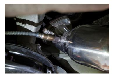
15. Remove the rear-most (2) bracket clips securing the rear oxygen sensor cables to allow it to reach the new sensor position.
