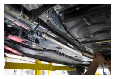
14. Install front oxygen sensors (closest to the flanges).
