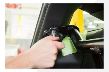
14. Re-install the seatbelt covers and remove the protective tape.
