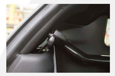
15. Using a 5/16" hex wrench, install the supplied shoulder harness collars.
