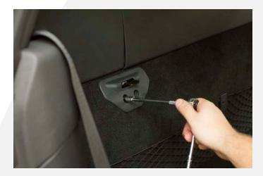
6. **458 ITALIA ONLY:** Using a 3mm hex wrench, remove the (2) fasteners securing the child seat restraint cover panel.
