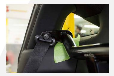
12. Position the support bracket on top of the child seat mounting tab and insert the supplied 13mm bolt. Tighten using a ratcheting wrench. (*NOTE: You can also use a 13mm socket, but it's difficult due to the space constraints. Due to the slight variations in vehicles construction, it may be necessary to remove the child seat restraint bracket in order to get the harness bar support positioned correctly before re-installing the restraint bracket.*)
