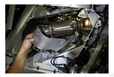
9. Using a 13mm socket, loosen the v-band clamp securing the factory header to the factory catalytic converter.
