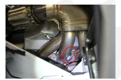
7. From the top of the engine bay, remove the (2) 5mm Allen bolts securing the EGR valve assembly to the engine valve cover.
