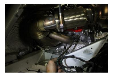
11. Remove factory header from vehicle.
