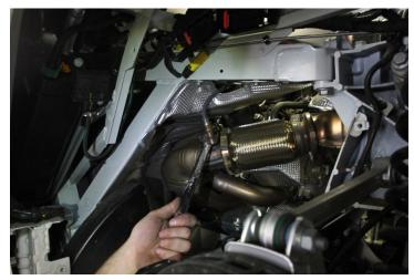
5. Remove the (21) 10mm bolts (17 short & 4 long) and the (4) T30 Torx bolts securing the rear under panel, and remove the rear under panel. (NOTE: Depending on the configuration of your lift arms, it may be necessary to put the rear wheels back on and lower the car to fully remove the panel.)
