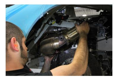
12. Install Fabspeed header onto the factory header studs.
