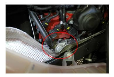
8. Using a 5mm Allen bit, remove (6) bolts securing the two-piece heat shield behind the factory header. Remove both sections of heat shield.
