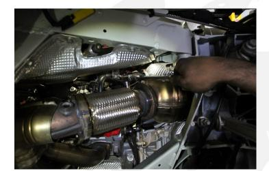
10. Using a 12mm socket, remove the (8) nuts on the header flange studs.
