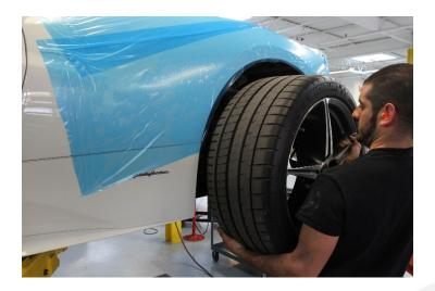
3. Using a 4mm Allen bit, remove the (14) bolts securing the front and back sections of the fender liners. Remove both fender liner sections.
