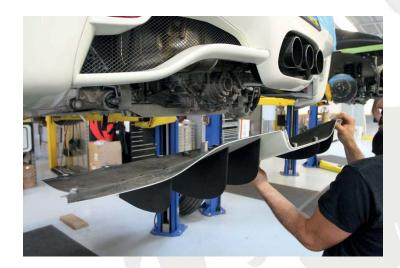
13. Reach up through the bottom of the rear bumper, above the exhaust tips, and remove the (3) 4mm Allen bolts securing the vacuum line bracket to the bottom of the air box.
