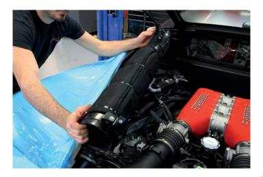
3. Using a 3mm Allen and 8mm wrench, remove the (2) bolts and nuts on the top of each side of the air box.
