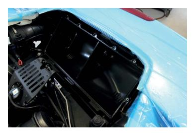
9. Using a flat-head screwdriver, loosen the hose clamp securing the intake elbow to either side of the air box.
