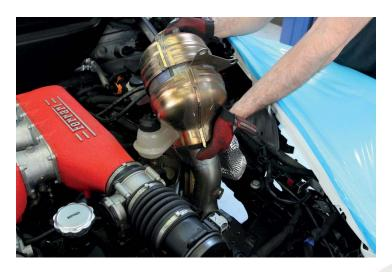
22. Slide the Fabspeed Sport Cat into the factory muffler inlet.
