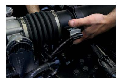
5. Using a T25 Torx, remove the (7) bolts around the edge of the air box cover.
