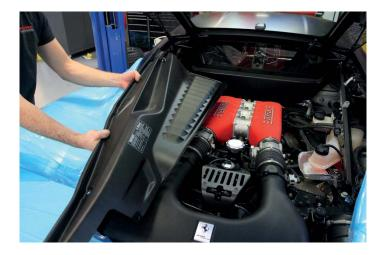
2. Using a 10mm socket and a flat-head screwdriver, remove the (2) bolts and the hose clamp securing each air intake tube and remove the tubes.
