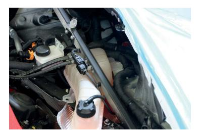
21. Slide coolant tank out of the way and carefully remove the cat. (NOTE: Heat shield will need to bend to allow for clearance. This can be repositioned.)
