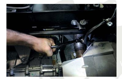
16. Remove the (3) 13mm bolts securing the cat bracket, and the (2) 13mm bolts running through the rubber damper bushings.
