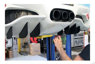
12. Remove the rear diffuser.
