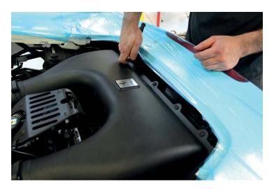
6. Remove the top section of the air box cover.
