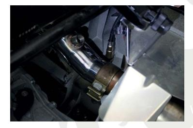
23. Align the Fabspeed cat and re-install the factory v-band clamp.
