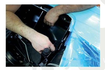
10. Separate and remove the soft rubber intake elbows.
