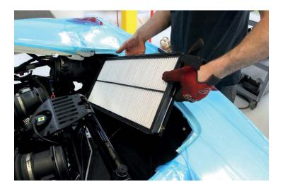
8. Using a 10mm socket, remove the (4) nuts securing the bottom section of the air box.
