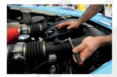
4. Remove the (2) similar nuts and bolts below each side of the air box.
