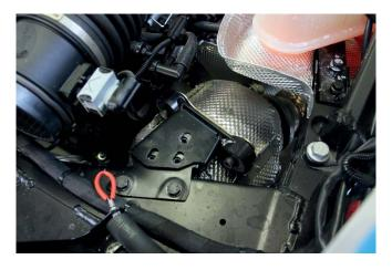
17. Remove (2) 4mm bolts securing the bracket to the cat heat shield and remove the heat shield.
