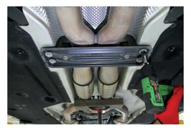
14. Remove the 18mm nut from each differential mounting bolt, slide the hanger bracket off each bolt, and replace the nuts.
