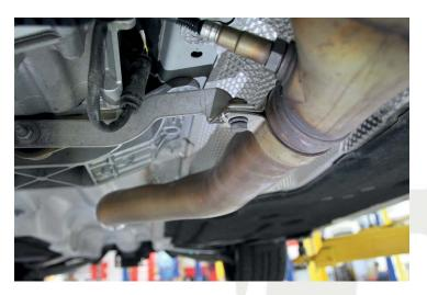
22. Using a 13mm socket, remove the center support plate from the factory x-pipe.
