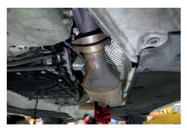
21. Re-insert the hanger bracket bolts, but do not tighten yet.
