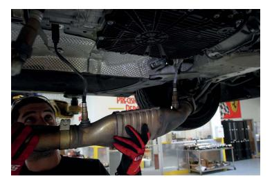
20. Re-hang the factory cats and insert and tighten the flange nuts & bolts.
