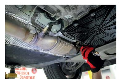
11. Using an E12 inverted Torx bit and a 14mm wrench, remove the (2) flange bolts from each side of the exhaust system.
