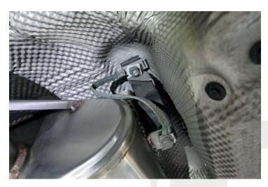
34. Re-attach the front hangers to the differential mounting bolts.
