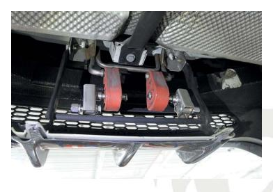
31. Remove the factory side muffler brackets and grounding straps and re-install on the Fabspeed mufflers.
