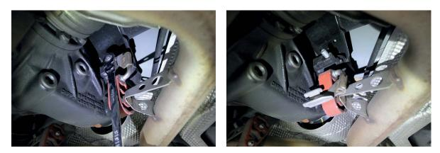
15. Remove the (2) 8mm bolts from the rear bumper support bracket and the (2) 13mm bolts from the top of the bracket.
