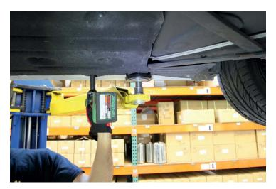
3. Remove the (2) 13mm bolts on either side of the rear subframe brace, near the rear wheels.
