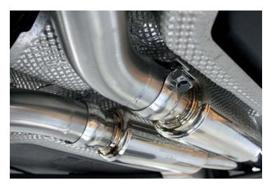
36. Slide tips onto muffler outlets, position, and tighten.
