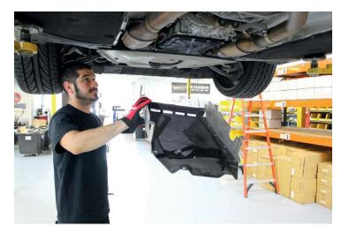
8. Remove the (6) 16mm bolts and (3) 10mm bolts securing the front skid plate. (NOTE: (2) of the 16mm bolts are located behind the front under panel. They can be reached with an open-end wrench without having to remove the under panel.)
