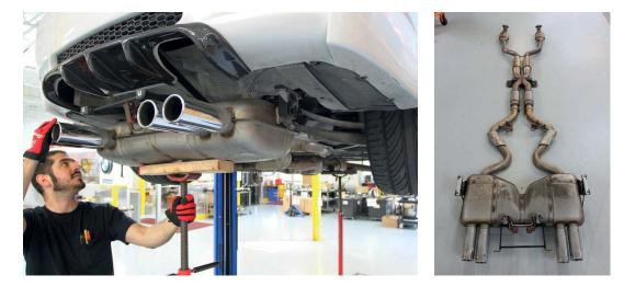
18. Using the method of your choice, cut the factory exhaust right behind the support bracket next to the secondary catalytic converters (See red line below).
