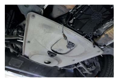
9. Remove the 16mm bolt from the center of skid plate and remove the plate.
