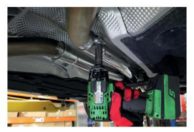
27. Using a 13mm socket, tighten the hanger bracket bolts.
