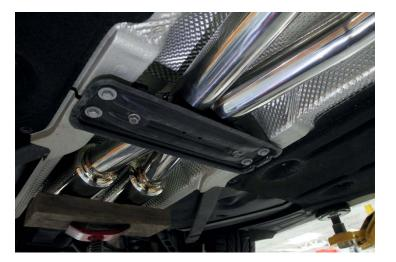
26. Using a 15mm socket, tighten the Accu-seal clamps.
