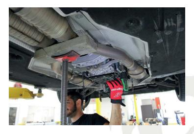
13. Remove the (4) 13mm bolts securing the center support plate.
