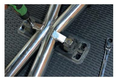
24. Hang the Fabspeed X-Pipe and slide it over the factory cat pipes. Slide the supplied Accu-seal clamps into position, but do not tighten yet.
