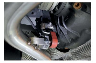
35. Tighten ball clamps using a 13mm socket.
