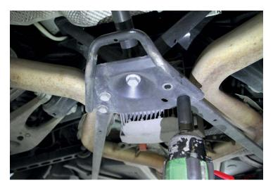
2. Remove the (2) 18mm bolts at the front of the rear subframe, on either side of the car.
