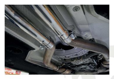
25. Re-insert the (4) bolts and secure the support plate into place.
