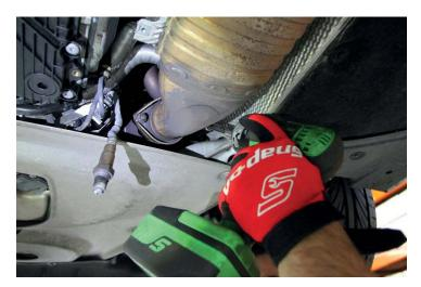
12. Support the center of the exhaust system and remove the (2) 13mm bolts from the front hanger bracket.
