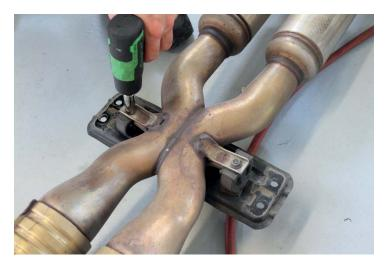
23. Re-install support plate on the Fabspeed X-Pipe.
