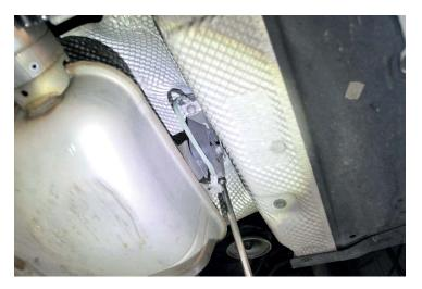
17. Lower full factory exhaust system from the vehicle.
