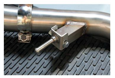
29. Remove the factory rubber hangers and install on the front of the Fabspeed mufflers.
