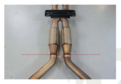
19. Pre-install the O2 sensors into the factory cat sections.
