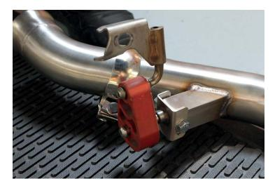
30. Remove the rear hanger bracket and hangers and re-install on the car. Insert Fabspeed rear hanger posts into the hangers.
