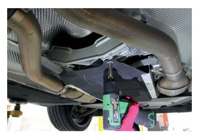
6. Remove the (7) 8mm bolts remaining around the perimeter of the center under panel.
