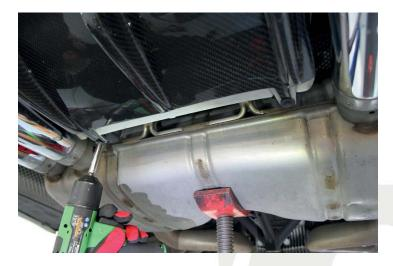
16. Remove the (2) 13mm bolts from each of the side muffler hanger brackets.
