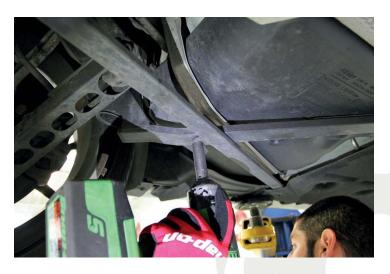
4. Remove the rear subframe brace. (NOTE: *This will come off in two pieces*.)
