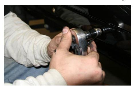
M. Tighten the bolt into the nutsert until it becomes snug in the rocker panel. DO NOT OVERTIGHTEN CAUSING THE INSERT TO SPIN!
