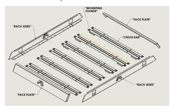
• Start by holding one "RACK SIDE" up above your vehicle. Use a ladder or platform that gives you good visibility of the roof. At this point you are making the first decision about where the "FEET" will land on the roof. Each set of 4 holes on the "RACK SIDE" represents the area that a "CROSS BAR" will be. "CROSS BARS" can be mounted with the "MOUNT FLANGE" facing forwards or backwards. (If unclear, or first rack consider a "dry" assembly of
