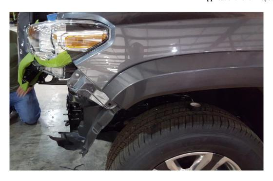
B. Mount bumper using OEM 14mm nuts. Do not fully tighten.
