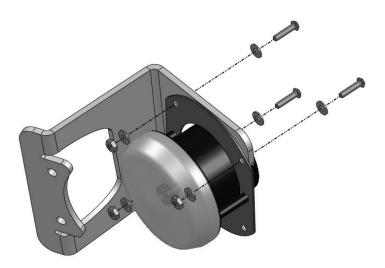
E. Install the fog light and bracket into the bumper using the remaining two holes available in the light insert. Use the 1-1/2" length  $\frac{1}{4}$ " stainless steel button heads with  $\frac{1}{4}$ " washers and nuts.
