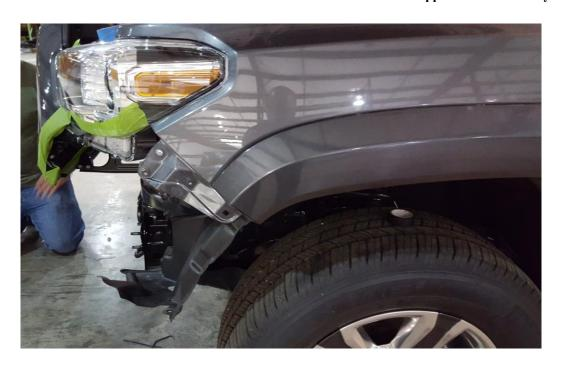
B. Mount brackets to truck using OEM 14mm nuts. Do not fully tighten.
