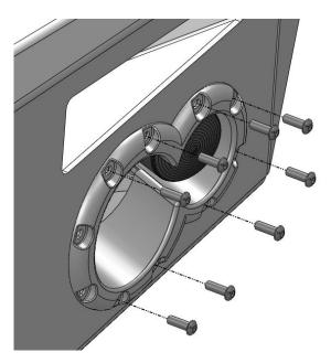
D. Install the Fab Fours fog lights onto the mounting brackets as shown below using the #8 button head screws, washers, and hex nuts.
