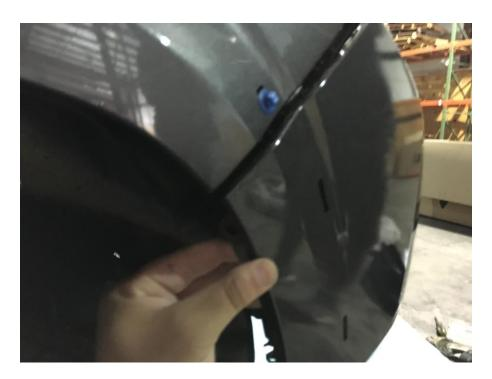
H. Remove 2 10mm bolts at the center bottom of bumper.
