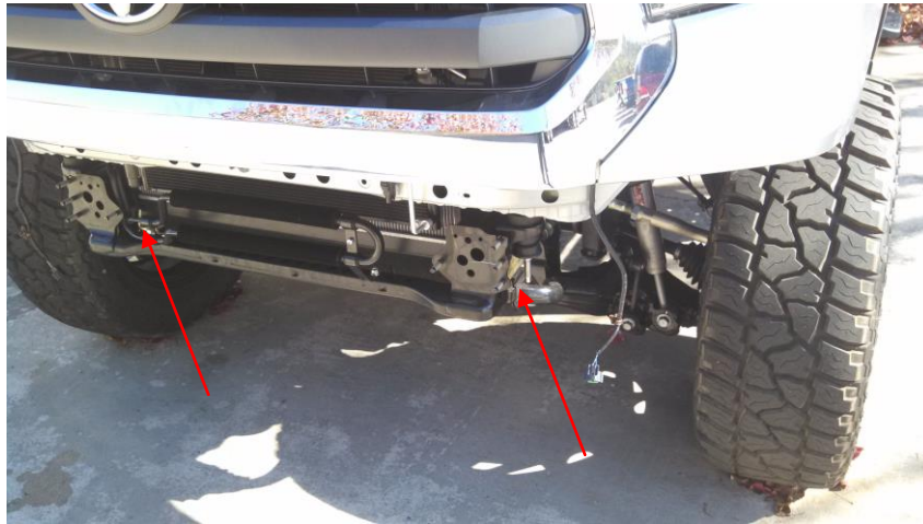
Figure 3 - Factory Bumper Connection
