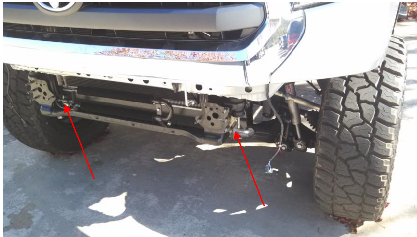
Figure 3 - Factory Bumper Connection
