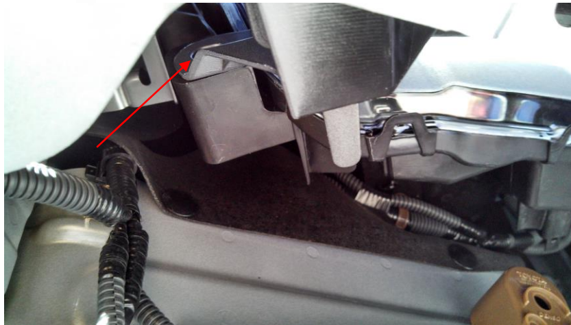
Figure 5 - Pop Clip Location Headlight to Plastic Fascia
