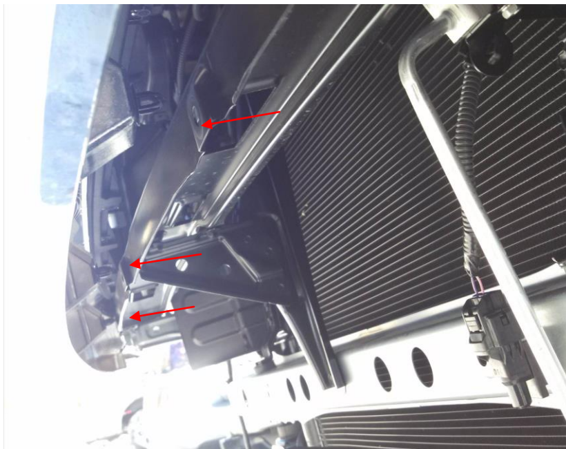
Figure 6 - Grill Plastic Clip Locations
