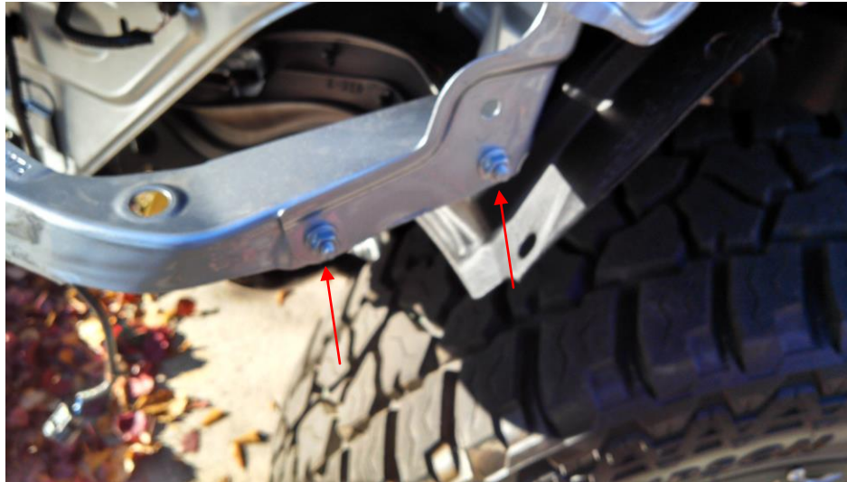
Figure 9 - Fascia Brace Nuts
