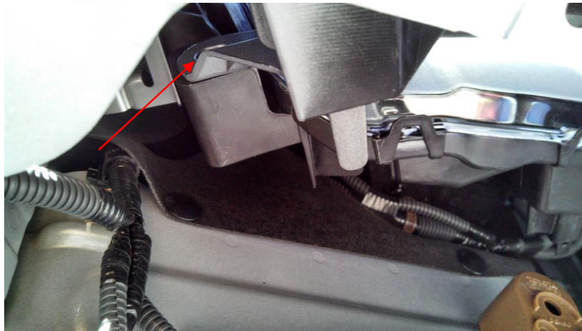
Figure 5 - Pop Clip Location Headlight to Plastic Fascia
