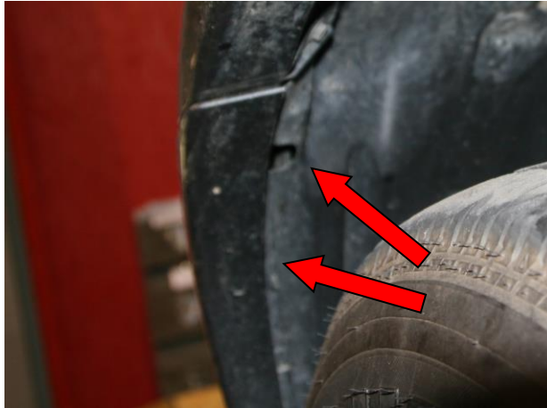
Figure 4 – Fenderwell fastener removal
