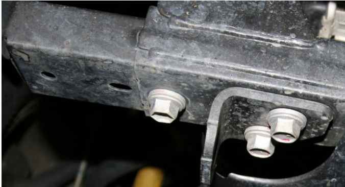
Figure 11 & 12 – Bumper beam extension and tow eye removal
