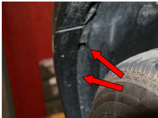
Figure 4 – Fenderwell fastener removal
