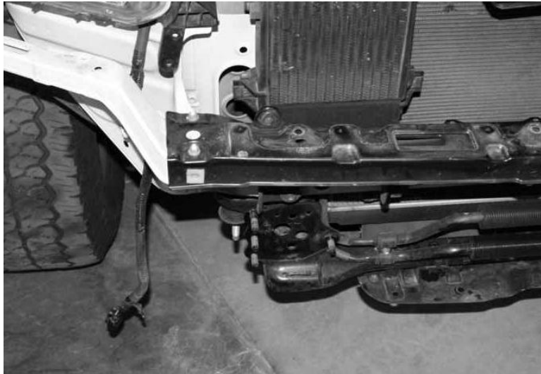
Figure 3 - Factory Bumper Connection
