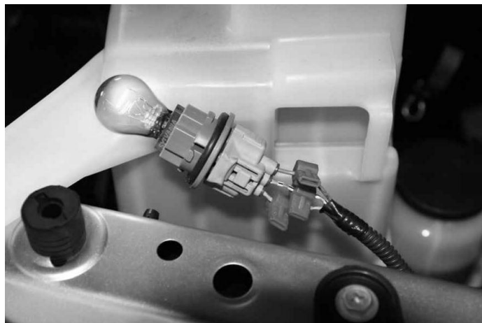
Figure 9 - Turn Signal Wiring Access
