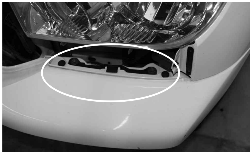
Figure 6 - Outer Fascia Fasteners
