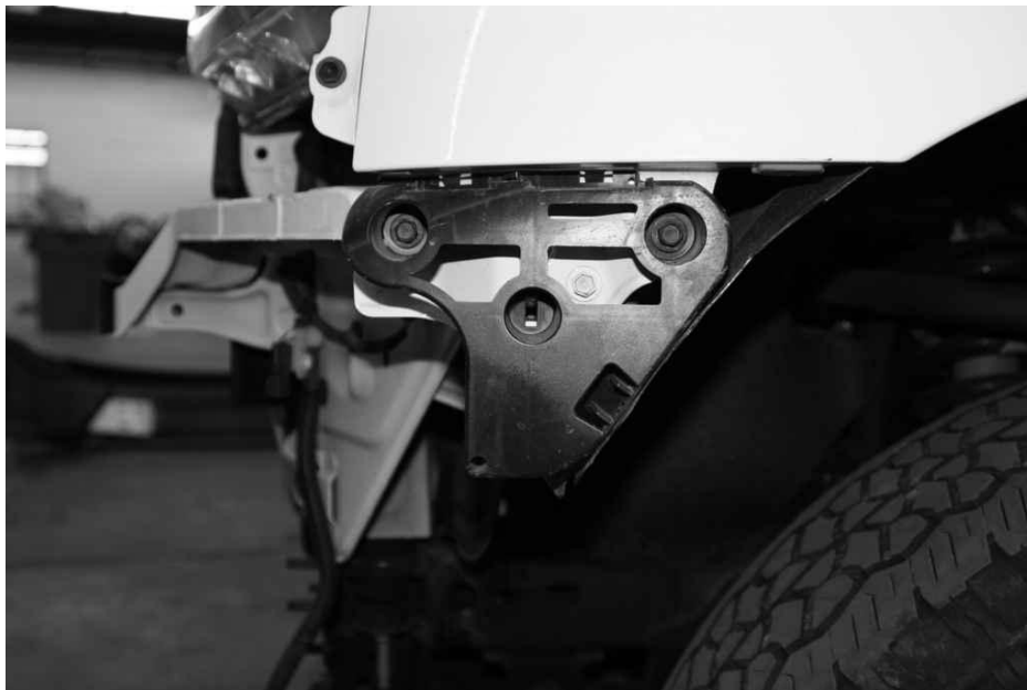
Figure 7 - Spacer Fastener Locations
