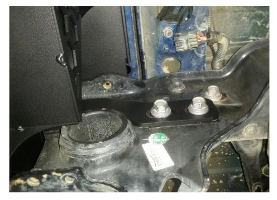
F. Align the bumper side to side and top to bottom to ensure a perfect fit to the truck. Allow for a 0.375" clearance to all painted surfaces if possible to allow for frame flex.
