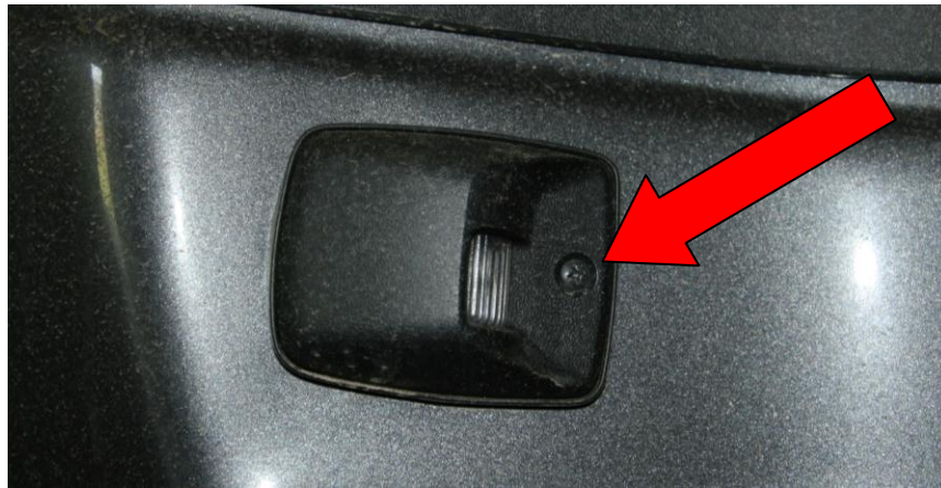
Figure 1 – License plate light removal
