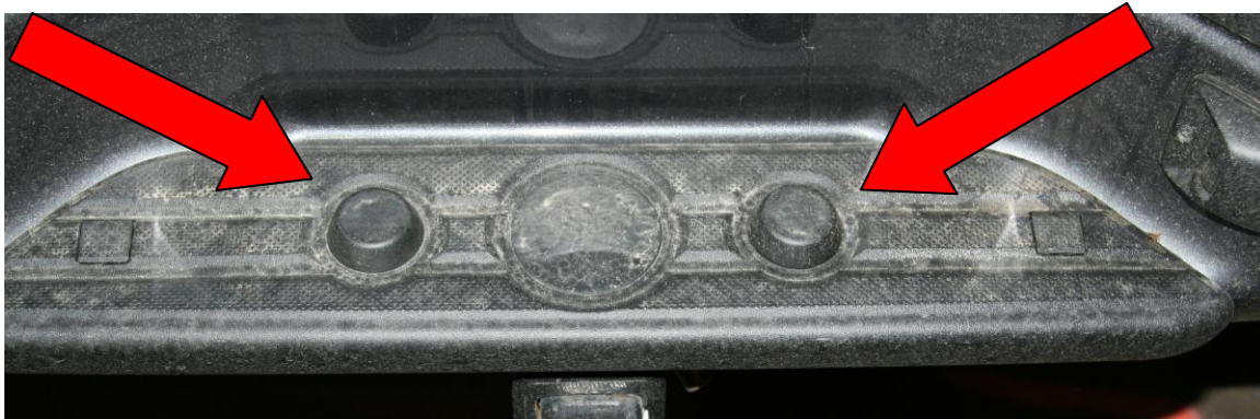
Figure 2 – Bolt cover removal
