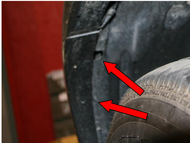
Figure 3 – Fenderwell fastener removal
