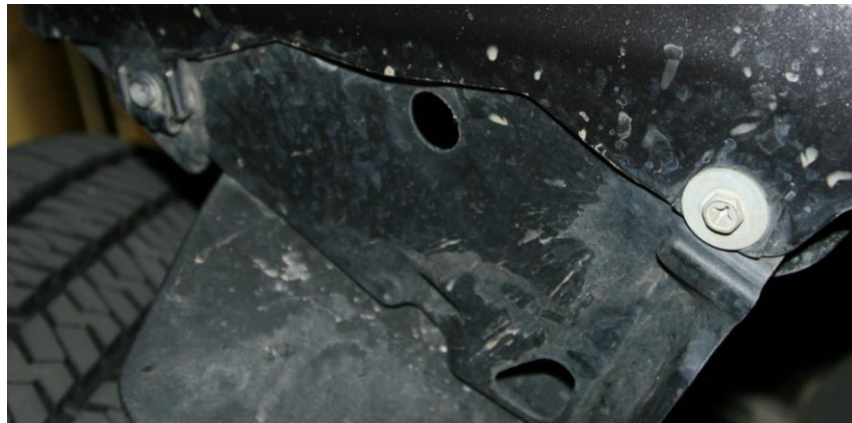
Figure 4 – OEM bumper cover screw removal
