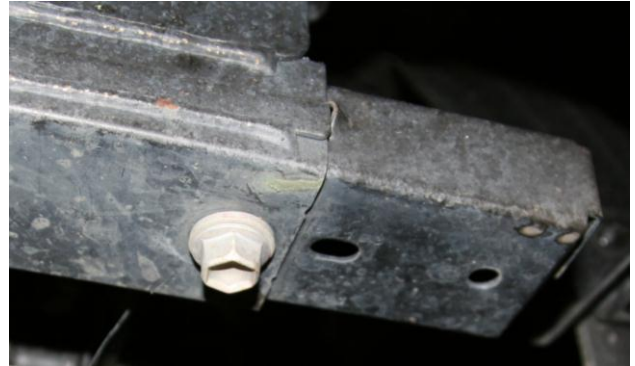
Figure 9 & 10 – Bumper beam extension and tow eye removal
