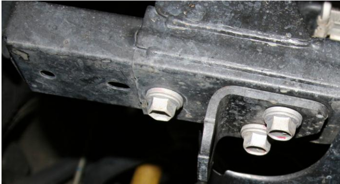
Figure 9 & 10 – Bumper beam extension and tow eye removal
