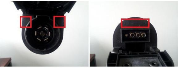
H. Secure all loose wiring and harnesses to the frame or bumper with zip ties. If necessary remove harness with trailer plug connector from OEM mount locations to allow for trailer plug connection.
