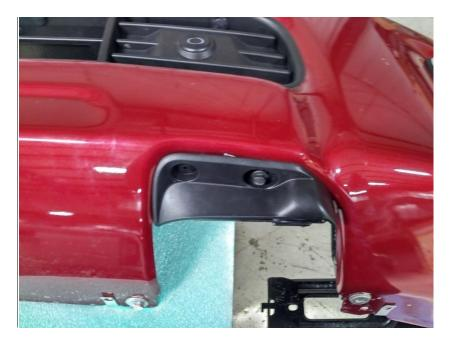
3. Remove center sensor mounting plates (may not contain sensor depending on trim level). If equipped with sensor unplug them from the harness
