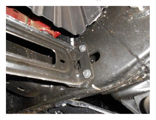
5. While supporting the bumper, unscrew the main bumper mounting bolts (3 per side) using a 14mm socket from the front face of the bumper and remove the bumper.
