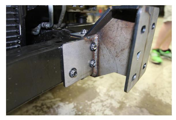
B. Mount bumper to bracket. With the help of at least two others and possibly a floor jack, to support the center of the bumper, lift the Fab Fours bumper into place. <u>Do Not Fully Tighten, Hand</u> <u>Tighten Only.</u>
