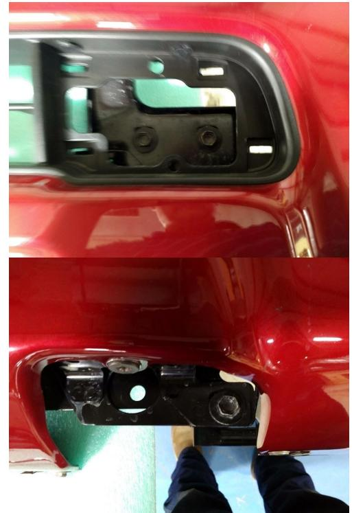
6. Remove the tow hooks using a 17mm socket or wrench.
